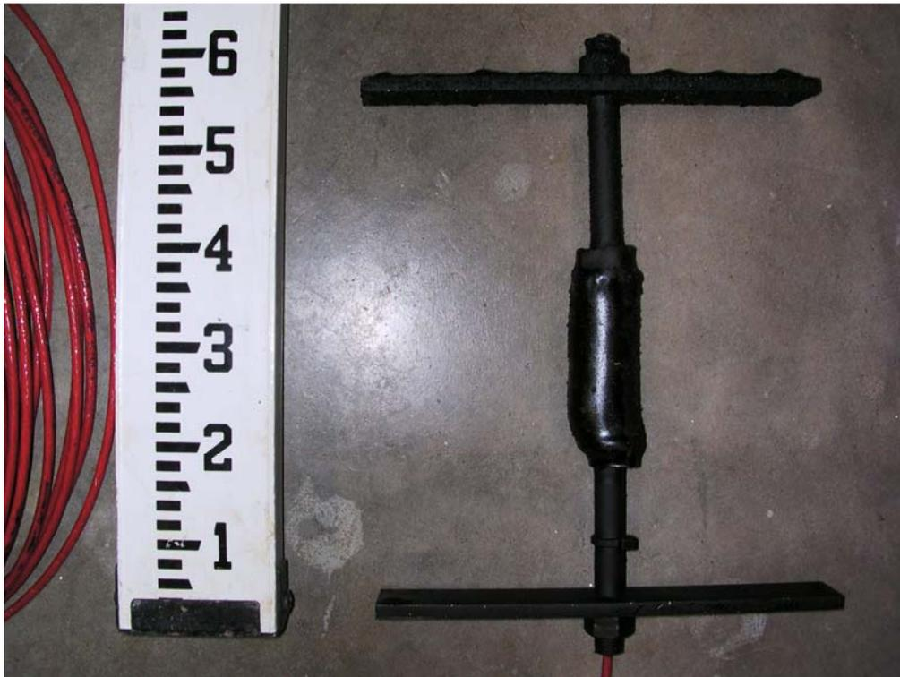
**Figure 4.7 – Asphalt Strain Gage**
