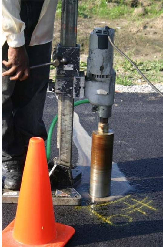
**Figure 7.7 – Asphalt Coring**
