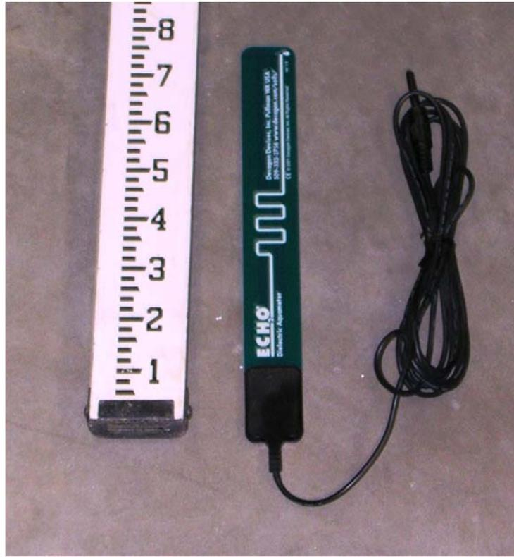
**Figure 4.18 – Moisture Content Probe**
