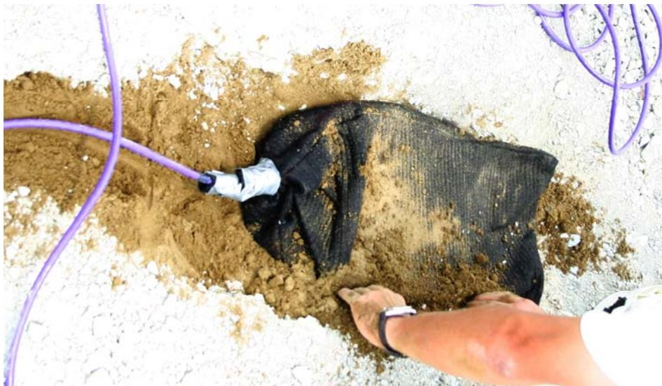
**Figure 4.24 – Placement of the Piezometer**
