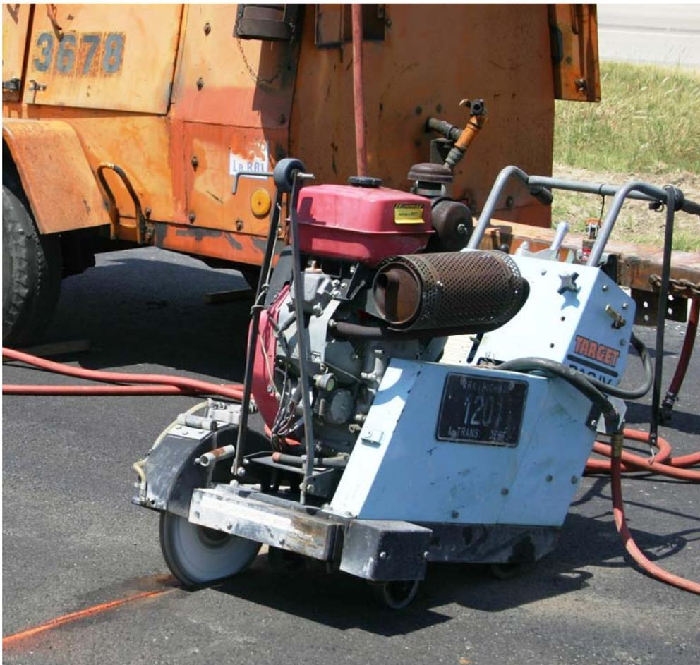
**Figure 4.27 – Pavement Saw**
