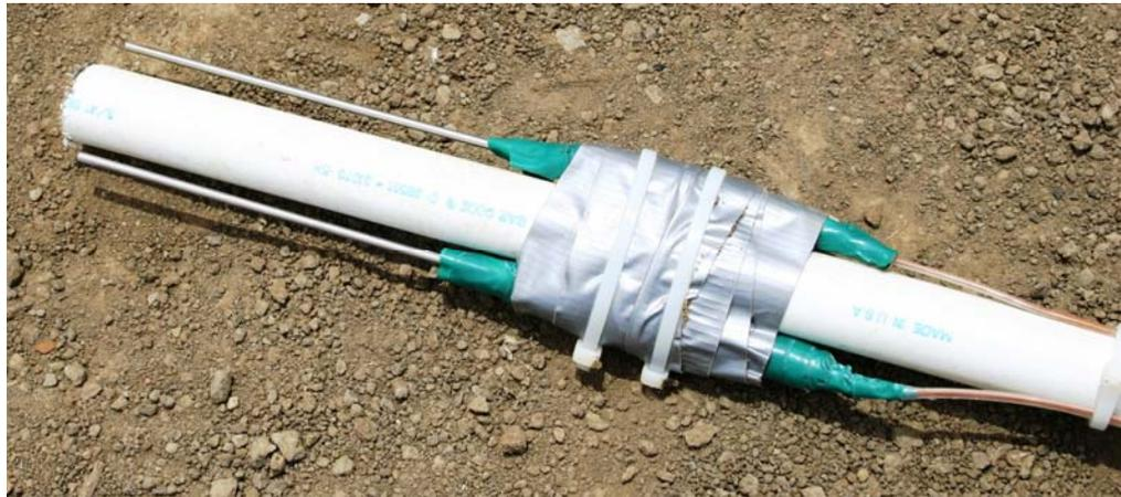
**Figure 4.15 – Subgrade Thermocouples Attached to a PVC Pipe**
