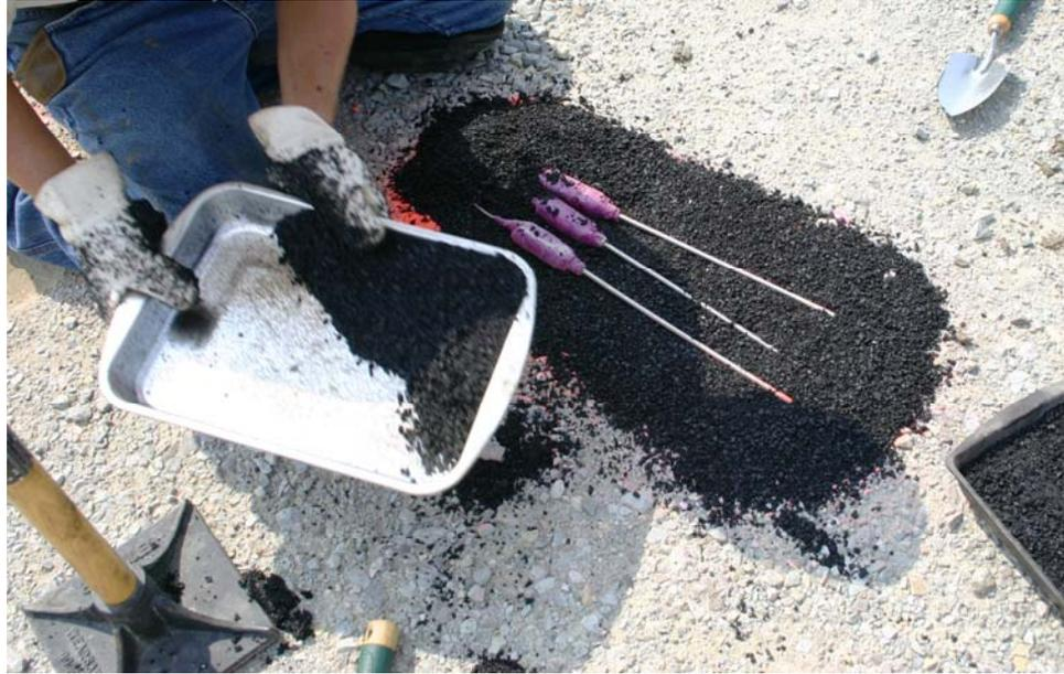
**Figure 4.17 – Asphalt Thermocouples**
