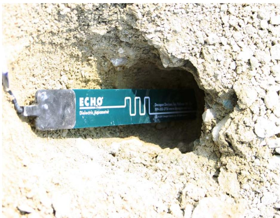
**Figure 4.21 – Insertion of Base Course Moisture Content Probe**
