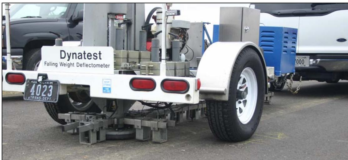
**Figure 7.2 – Falling Weight Deflectometer Test**
