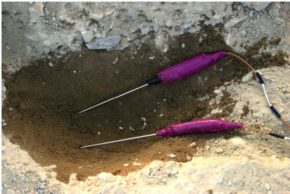
**Figure 4.16 – Base Course Thermocouples**
