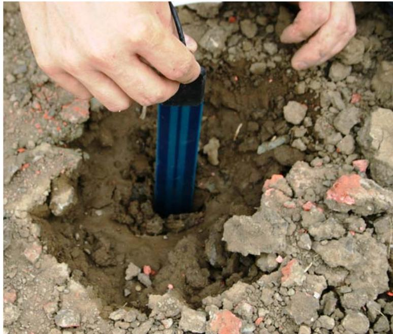
**Figure 4.20 – Insertion of Subgrade Moisture Content Probe**
