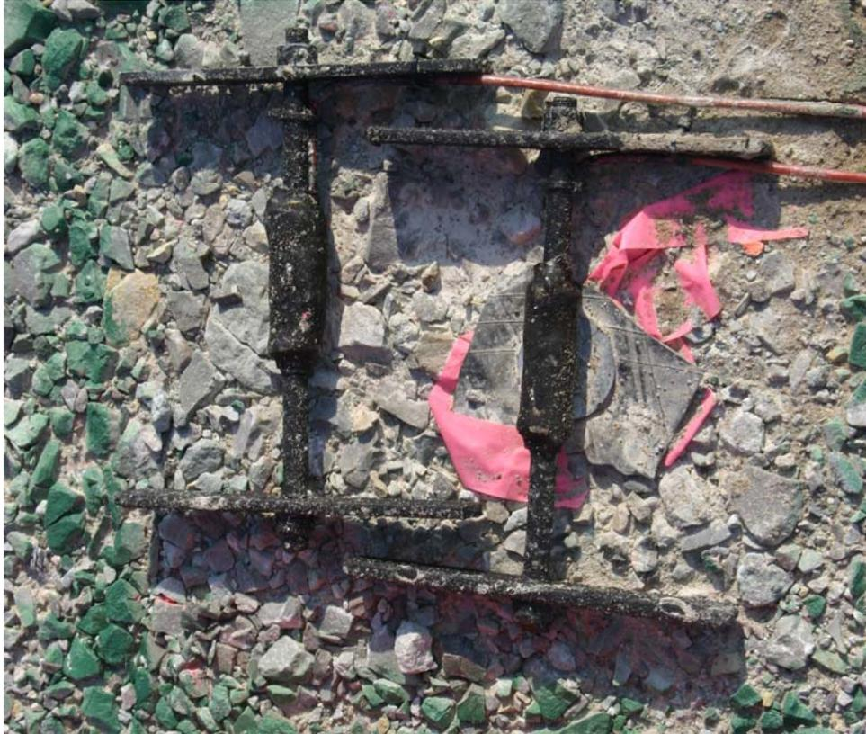
**Figure 4.8 – Asphalt Strain Gage Pair Prior to Paving**
