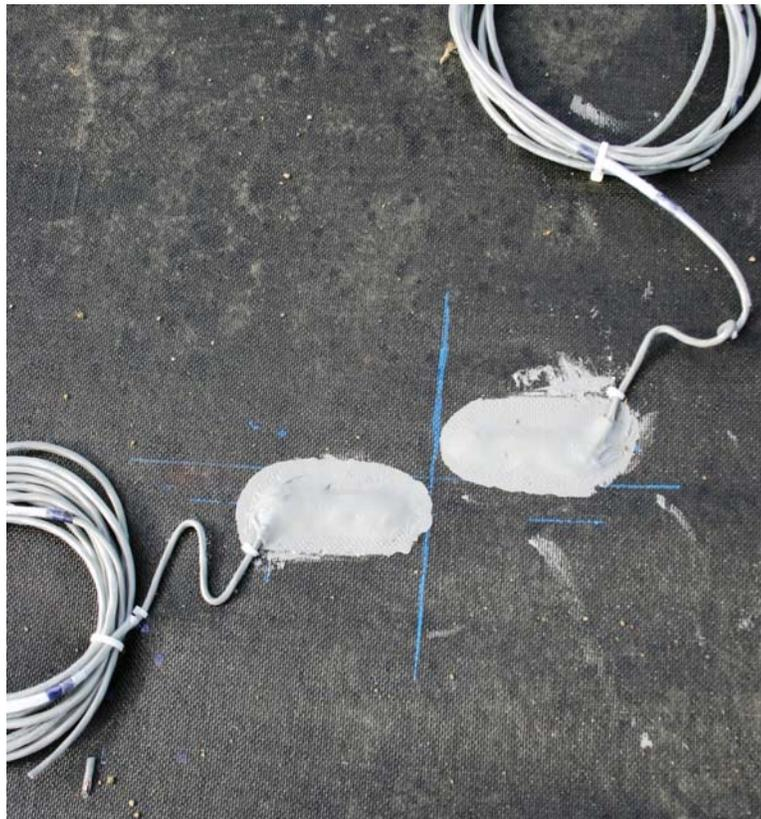
**Figure 4.13 – Geotextile Strain Gage in the Field**
