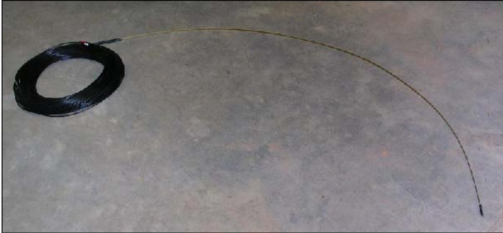
**Figure 4.26 - Piezoelectric Sensor**
