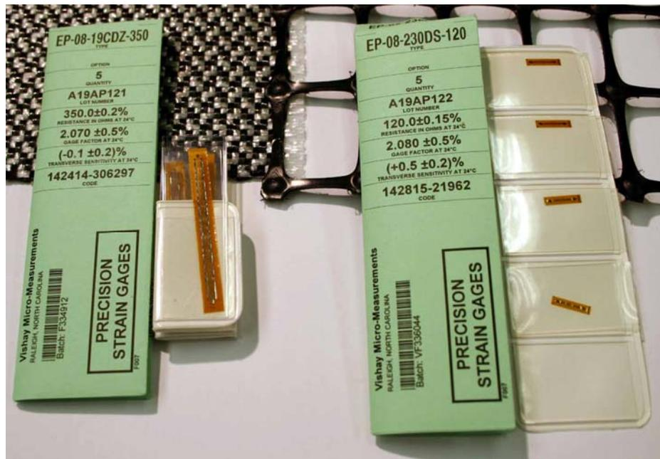
**Figure 4.11 – Foil Strain Gages**
