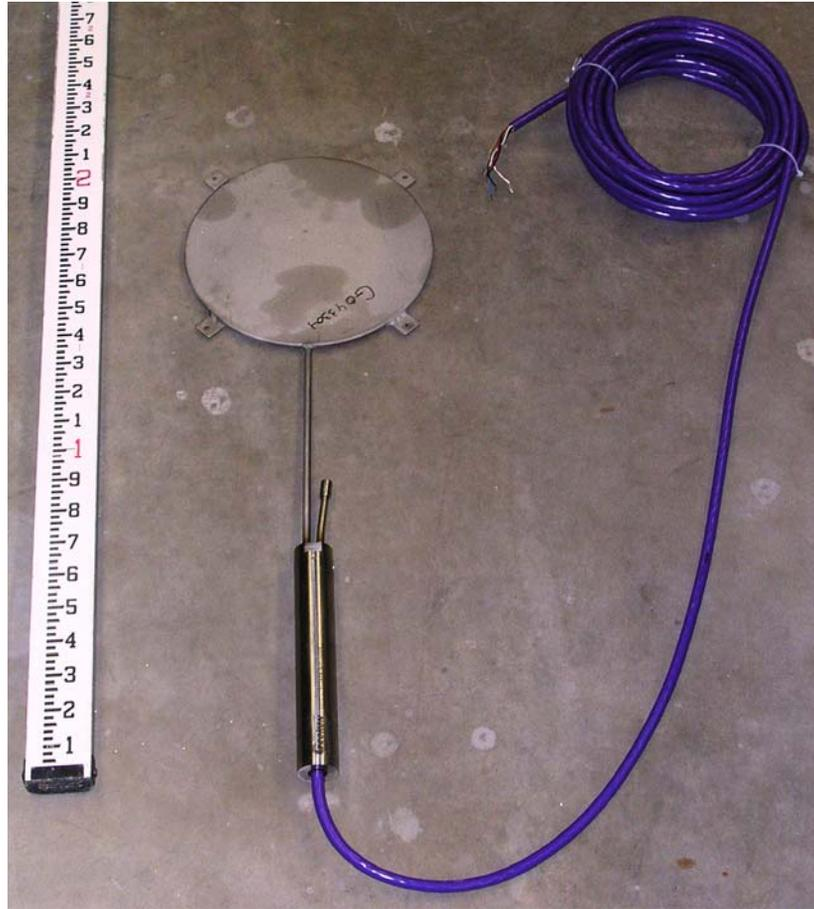
**Figure 4.2 - Earth Pressure Cell**
