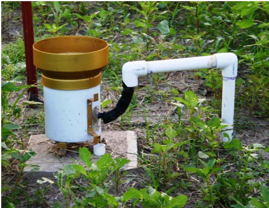
**Figure 4.25 – Installed Tipping Bucket**
